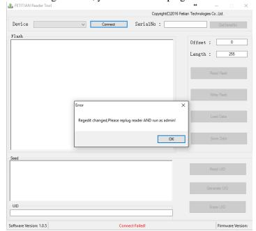
**Step #2**: re-plug reader and using administrator to run the tool again. And start to do operation. The tool provide three function, we will do introduction later.
