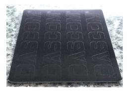
Real life DSML example. Security layer is appreciated tilting the card towards a light source
